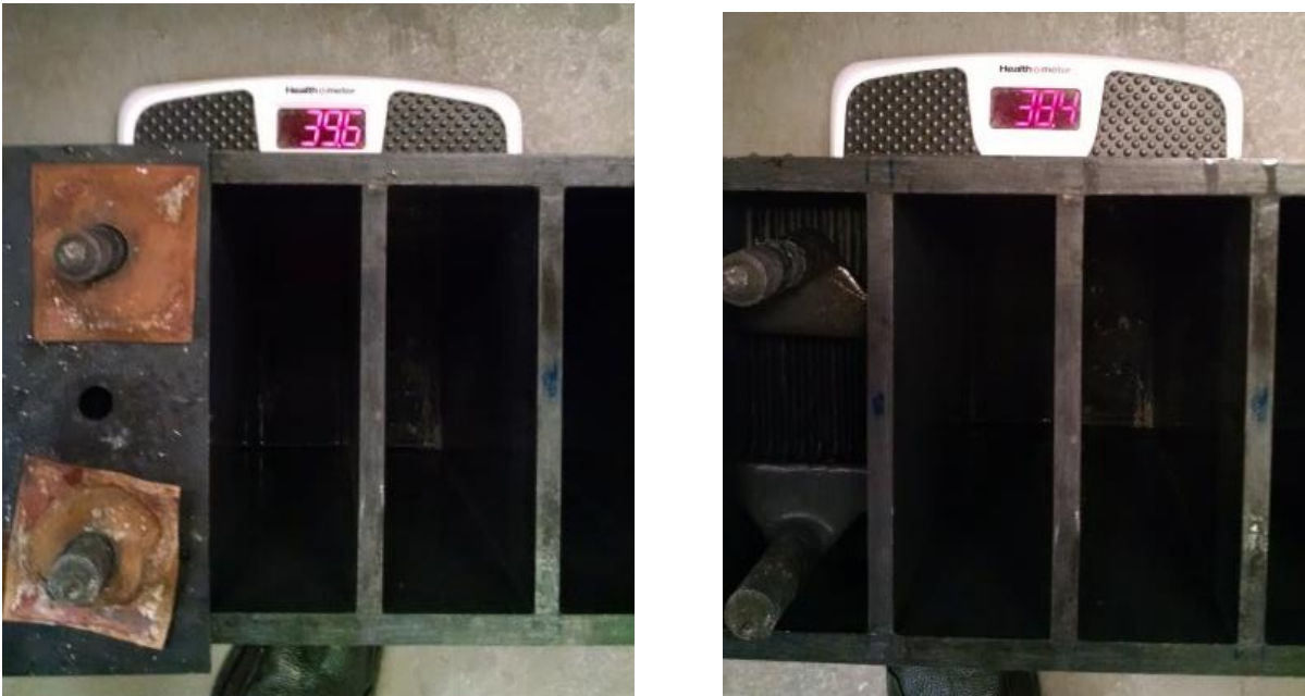
Figure 9. Apollo Energy Systems' GC1 battery is being weighed on a scale after being discharged. The electrolyte was not drained from a singular compartment that was being tested (left). The battery was drained of electrolyte only and reweighed (right).
