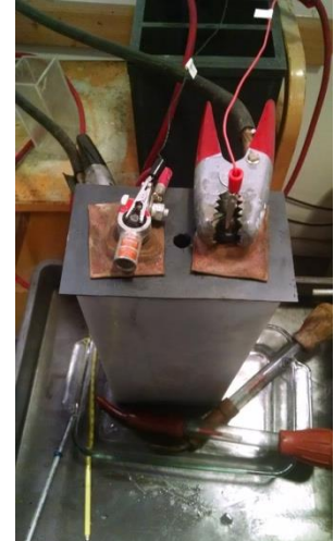
Figure 3. TPX1 with both the DataQ leads (small alligator clamps) and power supply leads (large alligator clamps) connected. The opening in the middle is for outgassing and measuring specific gravity and temperature.
