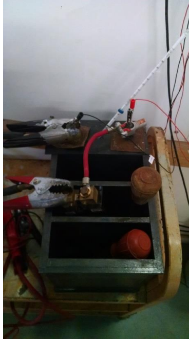
Figure 8. Discharge of a GC1 battery (Day 1). The two alligator clamps are shown here. The shunt is connected to the negative clamp again and then the shunt and positive clamp are connected to the terminals.
